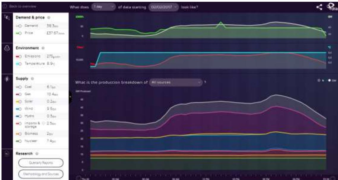
**Figure 1. Hourly electricity demand, price, environmental impact and supply of UK electricity (National Grid - Elexon, 2017)**
