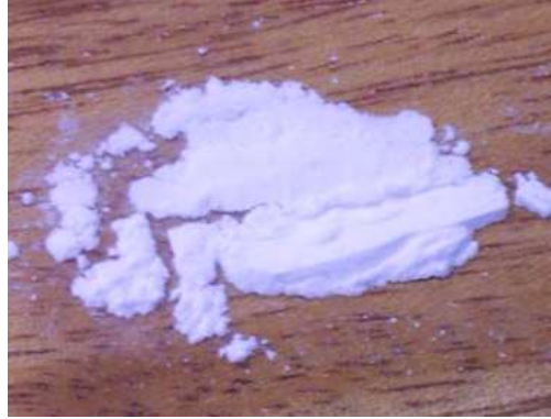
Figure: Micrencapsulated PCM commercialized by BASF
