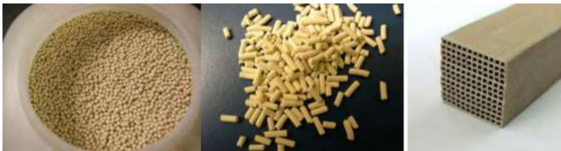
Figure: Examples of zeolite in different shapes and sizes: beads, pellets and extruded brick(SAIC)
