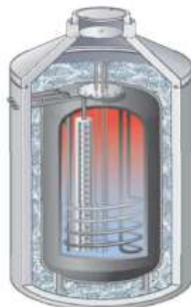
Figure: Mall, Mall-Pufferspeicher ThermoSol
