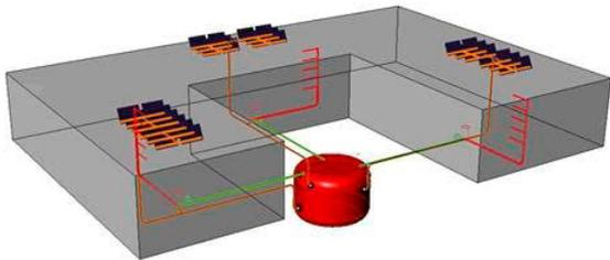
The proposed system is based on the **optimal combination** of hybrid photovoltaic-thermal solar panels (PVT), long term heat storage and heat pump use. These panels are a key element to achieve **self-sufficiency in buildings**, especially in dense urban areas where the roof availability is one of the most limiting factors.
